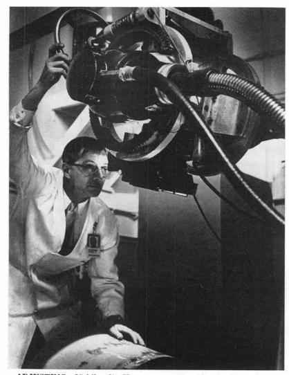
ADJUSTING 25-kilovolt X-ray generator, S. A. Ravenbyrne prepares to make an exposure of a large metal casting prepared by personnel of Sandia's Pattern and Foundry Section 4221-4.
